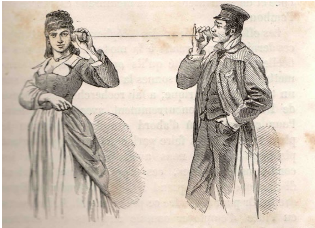
Fig. 2.2: The tin can telephone, or also known as lover's phone, connected two diaphragms with a taut string or wire, which transmitted sound by mechanical vibrations from one to the other along the wire.
